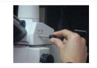
4. Focus the image in the microscope and then direct the image to the camera in order to see the image on the computer screen.
