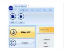
3. Press the **Analyze** button in order to see the live image on the computer screen.
