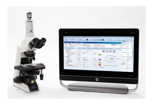
Motility & concentration, as well as droplets and coiled tails are rapidly and automatically analysed with SCA® Production.
